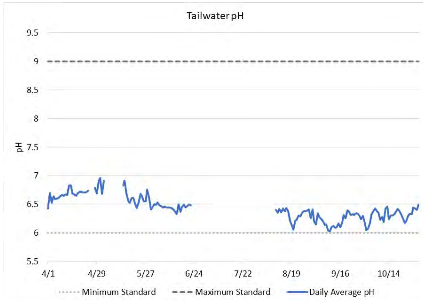
Figure 4-74.7 Daily average pH at the tailwater monitoring site, April 1 to October 31, 2021.
